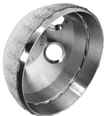
Figure 1. Jump cup with polar deflection, ribbed equatorial rim which gives an average oversizing of 1,000 microns (including coating). HaX-Pore®: double plasma-sprayed porous Titanium and Hydroxyapatite ( 500 \pm 50 \mu\text{m Ti} e 40 \pm 10 \mu\text{m HA} ).
