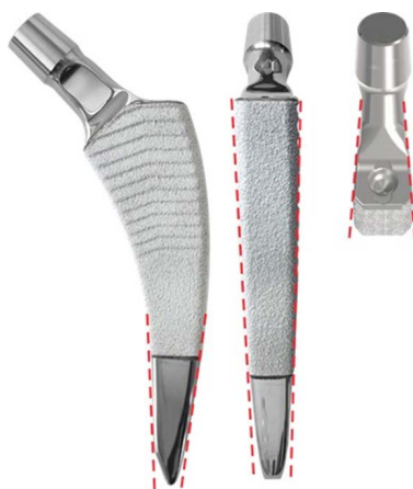
Figure 2. EXACTA RS triple tapered design with a double plasma spray coating HaX-Pore® in the metaphyseal region ( 300 \mu\text{m} pure Titanium and 50 \mu\text{m HA} applied with plasma spray technique. 12 sizes and lateral option.
