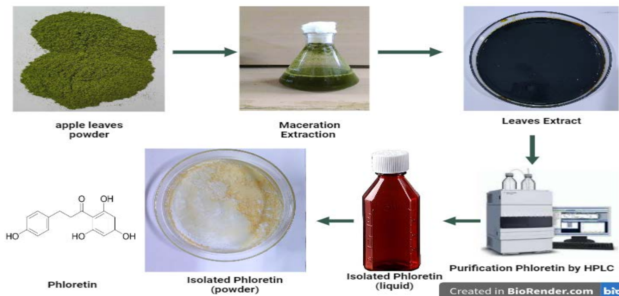
Figure 3. Purification phloretin procedure from Iraqi apple leaves.
