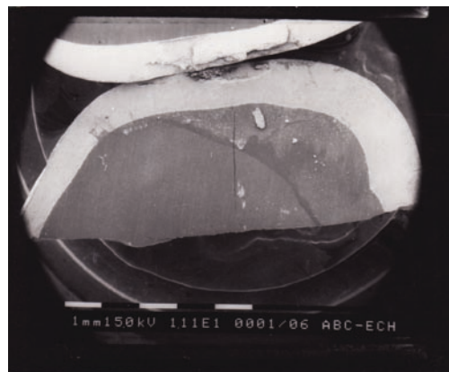
Fig. 5. Smear layers particles on the both sides of the failure site
